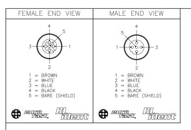
2. "/S2501" DESIGNATES RFID CABLE WITH PVC JACKET AND BLACK OVERMOLD.
